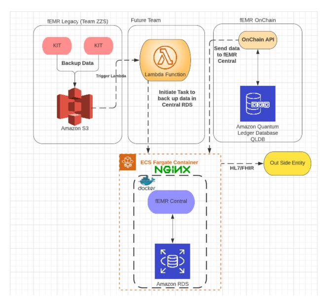
In this architecture, we will be relying on the internal service ecosystem of AWS to complete the flow of data from fEMR Legacy Kits to fEMR Central (which is supposed to be the centralized database for all the fEMR services). The uploading of data from kits to s3 should trigger a lambda function, which then initiates a task in ECS Fargate to process the data by giving instructions to docker image fEMR Central. Fargate will then run and store data in Central RDS.
